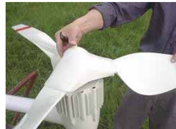
Fig.4.5 Fix wind turbine screw cover
