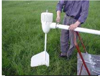
Fig.4.2 Fix wind turbine head assembly
