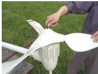
Fig.4.5 Fix wind turbine front cover
